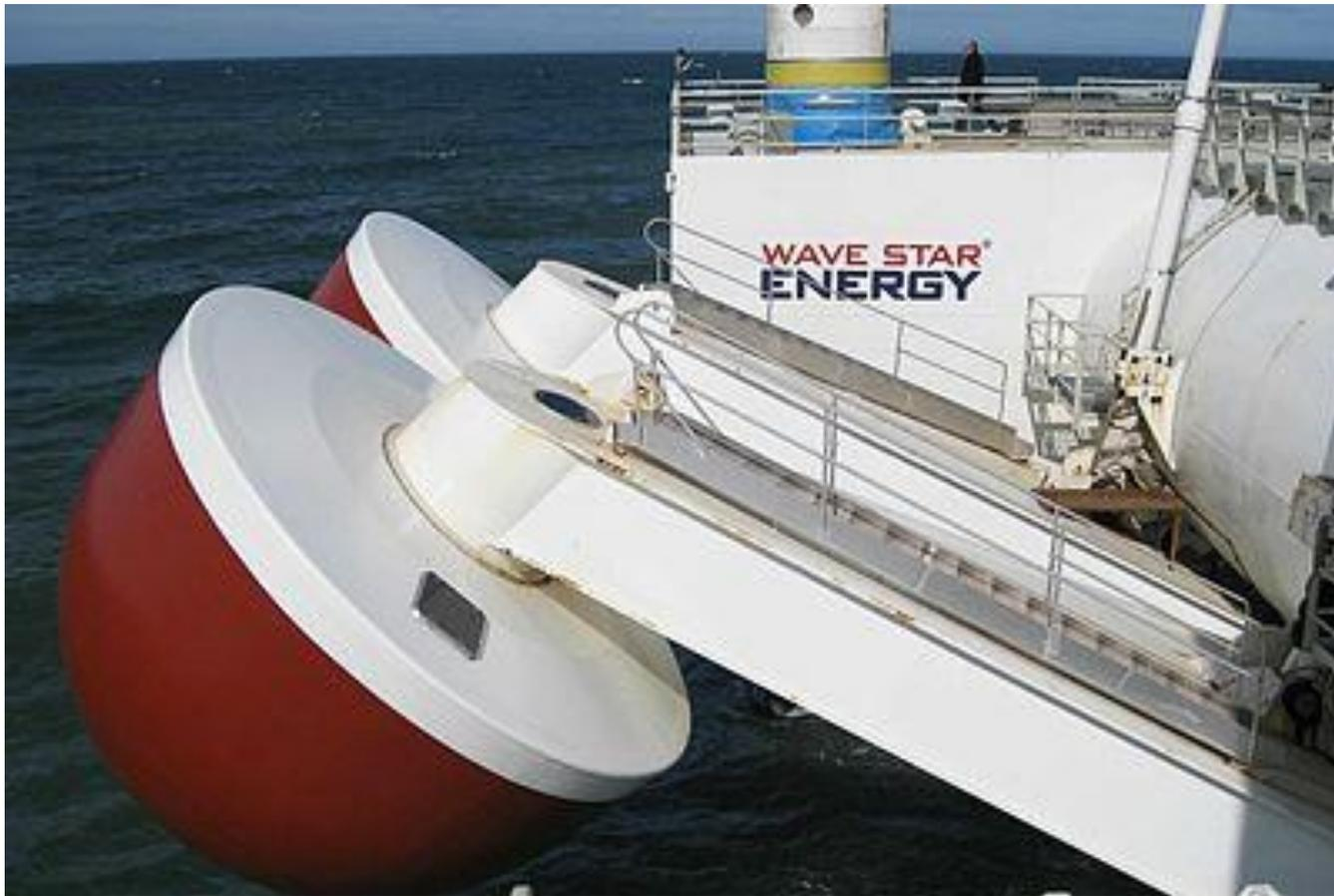
Revolute and spherical joints on the articulated arms and buoys.
